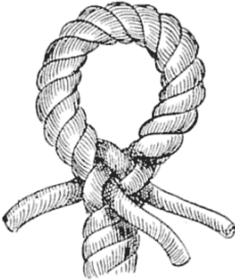
Illustration 8: The start of an eye splice
