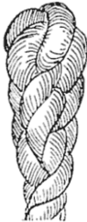
Illustration 7: Finished eye splice
